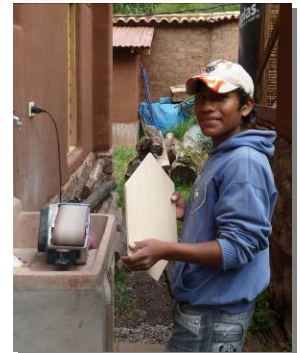
Julio prepares wooden filter lids used to protect the diffuser plate and to keep the biolayer clean.
